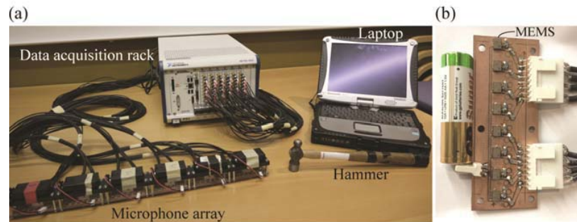
Figure 16: (a) All equipment needed to perform surface wave testing using the MEMS data acquisition system. (b) Close-up photo of a circuit board holding 8 MEMS microphones. An AA battery is shown as size reference.
